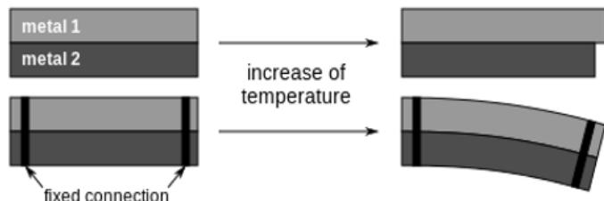
**By creating flexible connections between the parts, our shearless solution can reduce the impact of the bimetal effect.**
