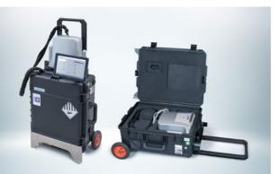
The Sparklike Laser Portable<sup>™</sup> is impressively compact and easy to handle. It can be easily used to measure noble gas content virtually anywhere.
